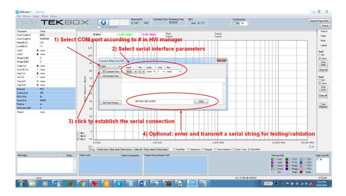
In order to automatically transmit test strings, they need to be entered into the desired segment file. You can add two serial command strings to each segment. Command SCPI\_A will be executed before the sweep of the corresponding segment. Command SCPI\_B will be executed after the sweep of the corresponding segment.
