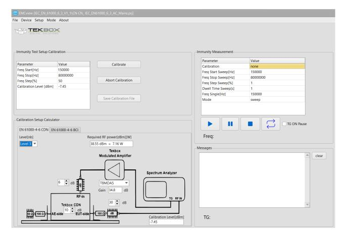
In order to run the immunity test, click the **Calibration** box in the **Immunity Measurement** window. Select the calibration file, configure the remaining parameters as desired and click the **start** button.
