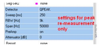
These settings are for re-measuring peaks (or doing a final scan as it is called sometimes). There is a chapter in the manual, explaining peak re-measurements.
