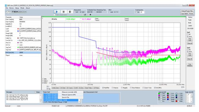
After the measurement of the five peaks is completed, the results of the quasi-peak measurement are displayed in the peak measurement box.
