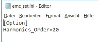
Save it as "emc\_set.ini" in the root directory where you installed EMCview. The above file will display 20 harmonic lines. The maximum number of harmonic lines is 99.
