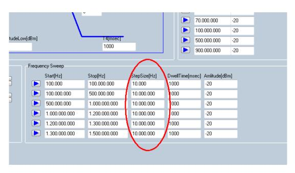
In order to change the step size to %, enter the **SETUP / OPTIONS** menu. In **MISC**, tick the % sweep box:
