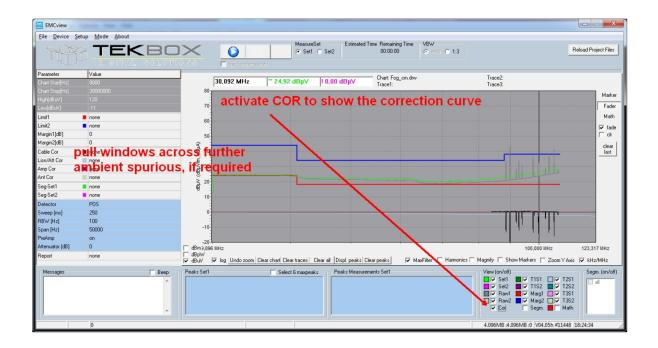
In the **File** menu, save the zero-compensation curve and thereafter load the zero-compensation curve. Disable the **Cor** box, if you want to make the compensation curve invisible. Then re-measure with the **Use Compensation** box under the **Play** button enabled.
