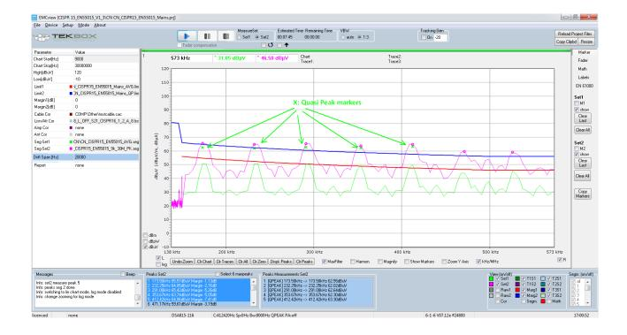
The next screenshots looks at the frequency range around 15 MHz and selects the highest point by manually placing a marker. First, pressing the **Clr Marker** button deletes the automatically generated markers. Next a manual marker is placed at the graph and then transferred into the peak list:
