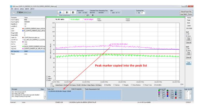
Finally, a QP measurement is carried out, selecting the peak in the peaks list, right mouse button and selecting Measure (consider drift). After the measurement, the QP measurement result appears in the graph window and peak measurement list. The result is at the same frequency, which shows that the spurious maximum has not drifted.
