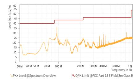
In the legend of the screenshot you can see QP limits, but the measurement was carried out using the peak detector. Peak detector measurement results are far faster than QP measurements and Peak detector
