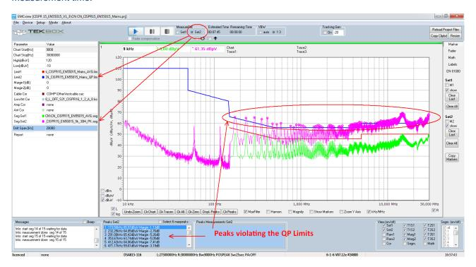
The result shows many peaks violating the QP limits. As explained in chapter 19, measurement results of the Quasi - Peak detector are always lower or equal compared to the results of the Peak detector. Consequently, there is the chance, that the spurious still may pass the QP-Limits, if measured using the QP detector.
